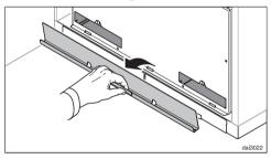
Remove the cover. It is held in place by magnets.
